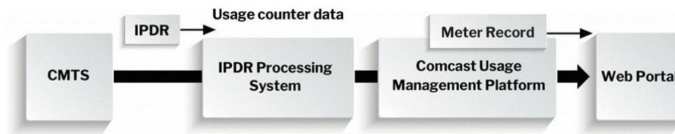
**Figure 4 - How the Meter Data Is Processed**
