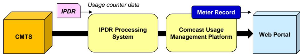
**Figure 3 - How the Meter Data Is Processed**
