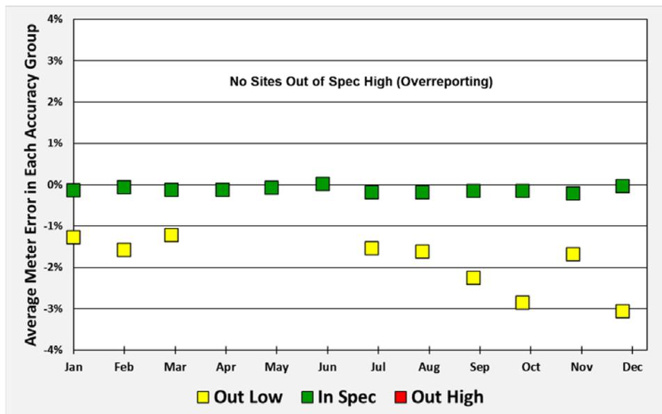
**Figure 7 – How Much Sites Were Within/Out of Spec**
